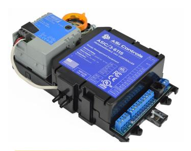
The five 24 Vac TRIAC outputs are ideal for driving contactors and relays. The analog outputs are used for modulated actuators, electronic pneumatic transducers, variable speed drives and other analog signal devices. The eight universal inputs counting pulses, monitoring contact closures directly, and for reading 4 to 20 mA, 0 to 5 Vdc or 0 to 10 Vdc input signals.
